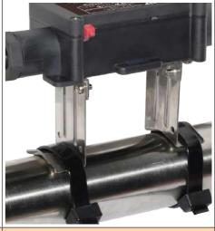
1: Two built-in <u>tabs</u> for mounting on a flat wall.
