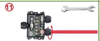
11: Slide the flat cable gasket into the cable gland and tighten the nut. Maximum torque 3Nm. Connect any other cables and close the lid.
