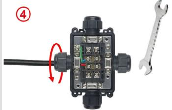
4 : Slide the round cable seal into the cable gland and tighten the nut. Maximum torque 3N.m.
