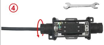
Slide the ground wire under the ground terminal square washer and tigthen the screw. Recommanded torque 1.6 Nm.
