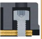
1: Anti-vibration blocking of the terminal block screws, resistant to thermal cycles.
