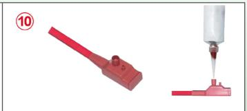
10: Place the assembly on a horizontal surface and fill with liquid RTV silicone through the filling funnel until this silicone begins to rise in the small degassing opening. Leave to cure for approximately 24 hours.
