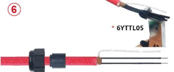
5: Remove the electric insulation sleeving on the requested length.
