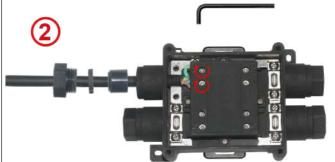
1: Remove outer jacket on 24mm. Then strip the conductors on 10mm. Eventually, crimp cable shoes. Slide the cable gland nut on the cable. Select the compatible diameter gasket and slide it too on the cable. 2: Put the neutral and line wires inside the screw terminals and tigthen them. Recommended torque 1.6 Nm.
