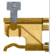
3: Terminal opening spring facilitating insertion and allowing possible replacement of heating cables.
