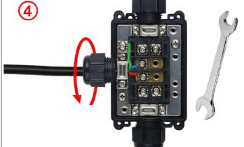
$\mbox{\bf 4}$  : Slide the round cable seal into the cable gland and tighten the nut. Maximum torque 3N.m.
