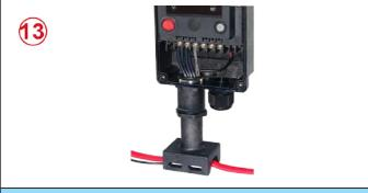
13: Connect the conductors and the temperature sensor according to the wiring diagram. Connect the power supply cable. Close the control box
