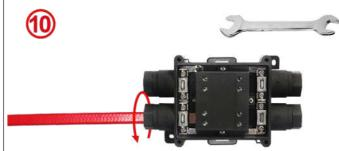
9: Tighten the terminal screw until electrical contact is made with the conductor of the heating cable. Tightening torque is around 1.5 Nm. This tightening torque may vary depending on the thickness and hardness of the material of the semiconductor thermoplastic compound. If necessary, check the continuity with an ohmmeter by measuring the resistance between the two terminals N and L.
