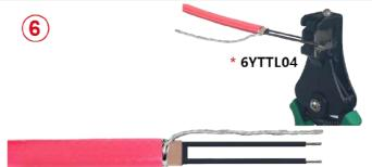
5: Cut and remove the heating section between the two bus wires on the requested length.
