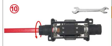
9: Tighten the terminal screw until electrical contact is made with the conductor of the heating cable. Tightening torque is around 1.5 Nm. This tightening torque may vary depending on the thickness and hardness of the material of the semiconductor thermoplastic compound. If necessary, check the continuity with an ohmmeter by measuring the resistance between the two terminals N and L.
