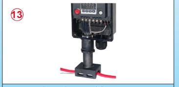
13: Connect the conductors and the temperature sensor according to the wiring diagram. Connect the power supply cable. Close the control box.
